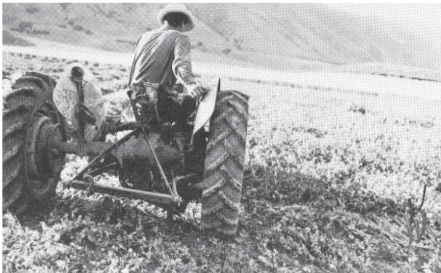
The farmer cuts his crop with a mowing machine. He does this by attaching a special part called a curler to the cutter bar. Look closely at the second picture to see this part. The curlers lift the vines up and turn them over. When the farmer cuts the next row, he does not run over the pods and mash the peas.
