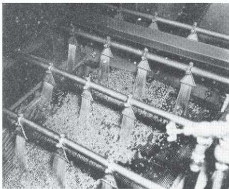
Then the peas are rolled over a metal screen. This sorts the peas. The holes in the screen are different sizes. Each size of pea drops through the screen at a different place.
