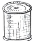
so air cannot possibly leak through. The cans have the bottom ends only applied. The cans and the top ends of the cans are sent to the buyers. After the food has been put into the cans, special machines seal the tops on the cans.
