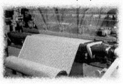
employ compressed air to insert the filling yarn across the warp. In addition to speed and versatility, another advantage of these modern weaving machines is their relatively quiet operation.
