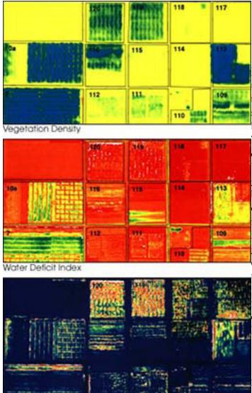
False color refers to a group of color rendering methods used to display images in color which were recorded in the visible or non-visible parts of the electromagnetic spectrum. These three false-color images were acquired by the Daedalus sensor flying aboard a NASA aircraft.
