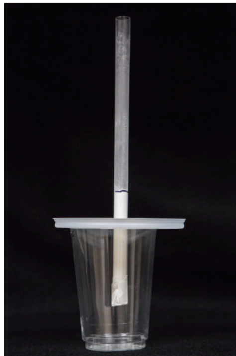
PHOTOGRAPH OF A COLUMN SETUP USING BABY POWDER AS A SUBSTITUTE FOR SILT. THIS COLUMN IS READY FOR WATER TO BE ADDED.
