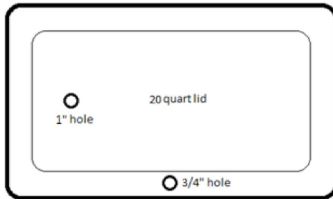
5. Drill a 1" hole near the top of one side of the 20-quart storage tub. This hole is for the pump cord and the water tube.
