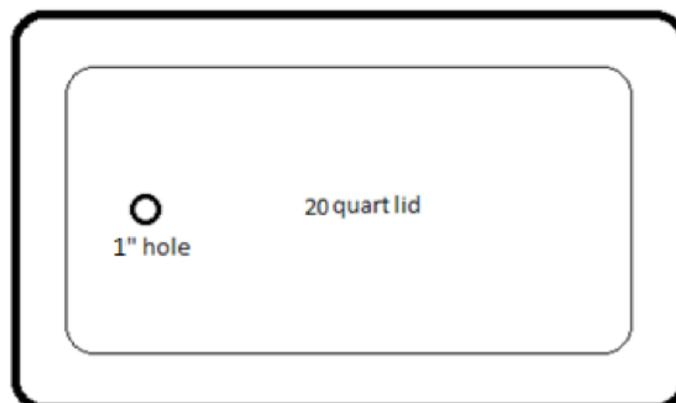
4. Drill a 3/4" hole approximately 1/2" from the edge of the lid or at the top of the front side of the 20-quart tub. This hole is for adding fish food.
