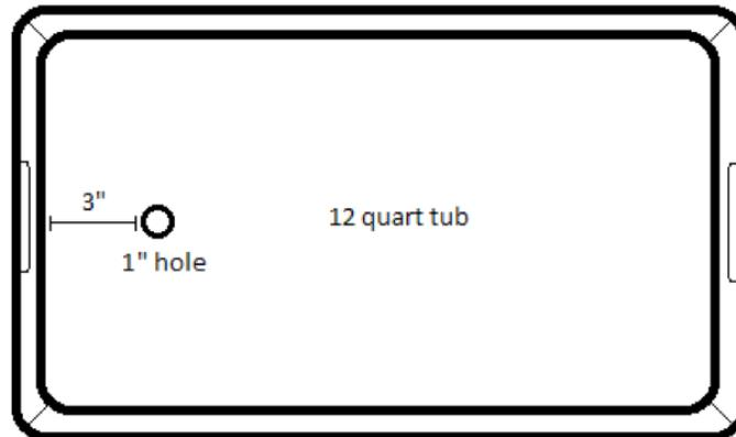
3. Drill a matching 1" hole in the lid of the 20-quart storage tub, such that the holes line up exactly when the 12-quart tub is nested on top of the lid. These holes are for the drain tube that will allow water to drain from the grow bed to the fish tank.
