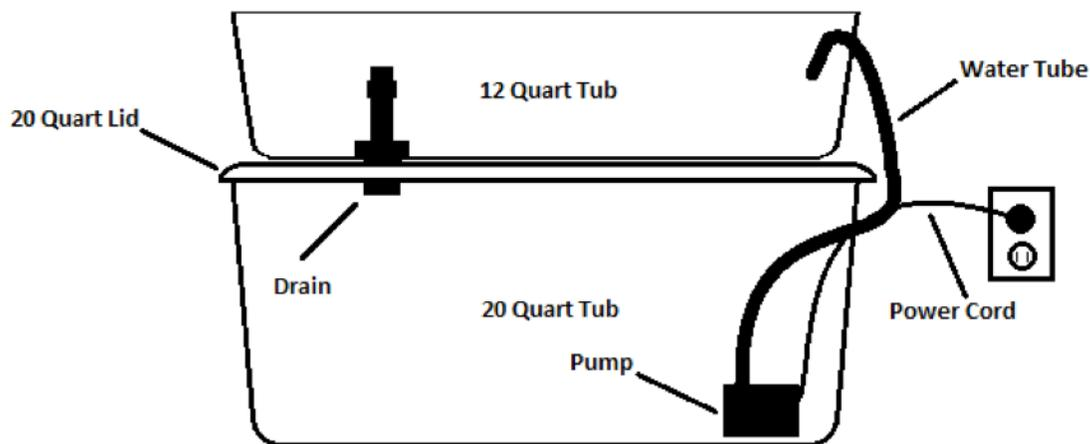
9. Fill the 20-quart tub about 3/4 of the way full of de-chlorinated water (approximately 15 quarts; see De-chlorination Procedure on page 9).
