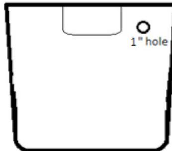
6. Drill a 3/4" hole near the top of one side of the 12-quart storage tub. This hole is for the water tube and must be located above the level of the drain tube.
