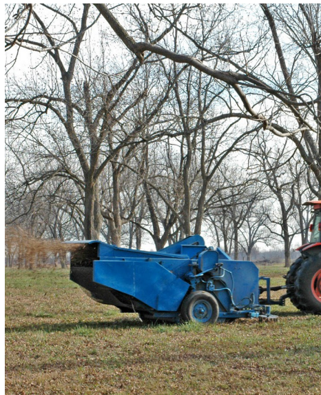
The harvester picks up the pecans and blows the sticks and leaves out of the way.
