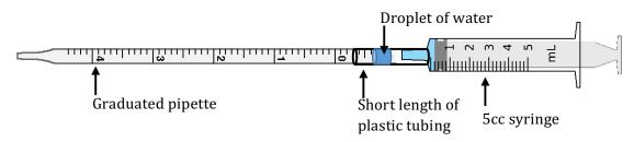
It may be beneficial to show students how to assemble the respirometer prior to starting the lab activity. Respirometers can stand upright on their own, however, if there are concerns about tipping over, the respirometers can be placed within a ring stand for stability.
