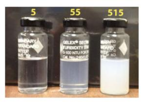
Turbidity is the measure of relative clarity of a liquid and can be used as an indicator of bacterial content. Presence of bacteria increases the cloudiness and therefore turbidity of the milk.
