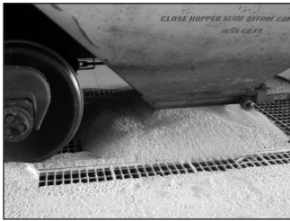
Receiving Grain by Railcar
