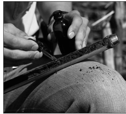
Field Testing for Soil pH
