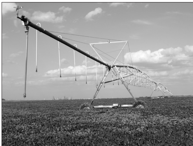
Center Pivot Irrigation with Drop Nozzles
